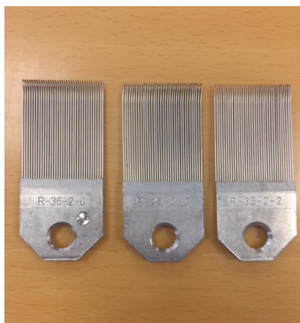
Plomos urdidor (1"). Comb leads for Warper (1").
